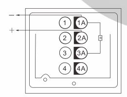
Connection Description: "\Theta" Positive power; "⊖" Negative power. Double light: Operating Voltage 9V~24V, according to the connection diagram, Red LED without lighting and Green LED flash means in the nomal work, break glass/press ABS panel, RED LED always lighting and Green LED no lightning means in the state of alarm.
